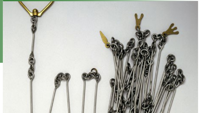
(Top) Magnetic compass. Courtesy Beltrami County GIS/Mapping (Bottom) Surveyor's chain. 66 feet in length with 66 1-foot links. Courtesy Beltrami County GIS/Mapping
