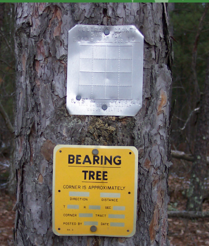
(Left) Corner Location Tags (CLT's) nailed to a bearing tree. Top silver one used by surveyors and foresters 1970-1985+-. Top one used 1985-Present+-. Photo by Neal Adams (Right) Original field note
